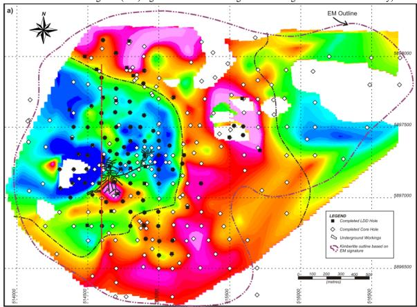
Figure 7-6 shows the EJF isopach map and highlights the thick deposits dominantly confined to the crater area of the kimberlite complex and attaining thicknesses in excess of 100 metres. Distal deposits occurring outside the crater are generally less than 30 metres in thickness.
