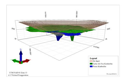
FIGURE 14-21 ORION SOUTH RESOURCE CONSTRAINING PIT
