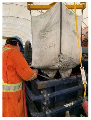
PLATE 2: BULK BAG BEING EMPTIED INTO THE ROM FEED BIN
