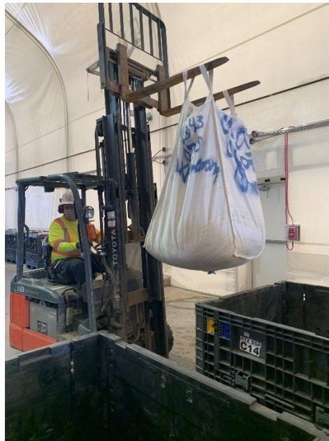
**PLATE 4: DMS CONCENTRATE BULK BAG BEING LOADED INTO SEALED PLASTIC CONTAINER**
