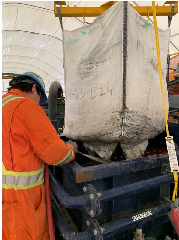
**PLATE 2: BULK BAG BEING EMPTIED INTO THE ROM FEED BIN**
